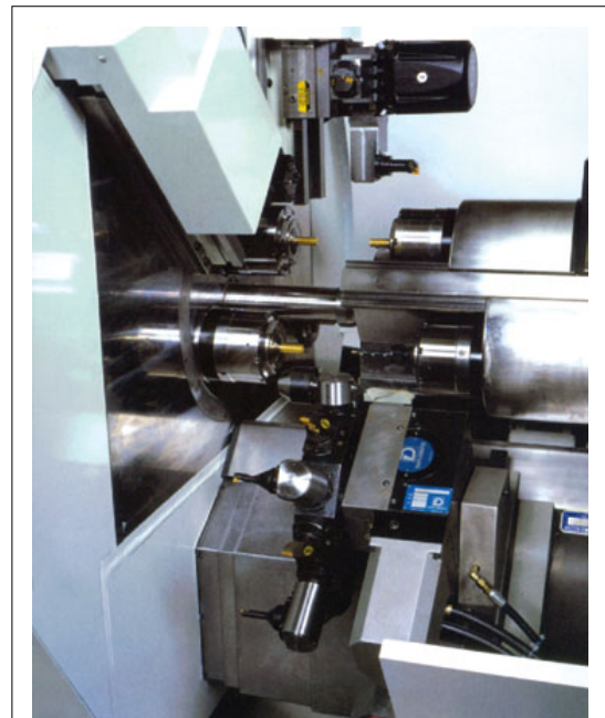
PHOTO FIVE CAPTION: Each of Tri-Turn's three main spindles is directly opposed by a counter spindle and is served by a live turret, providing a total capacity of 40 turning and rotary tools.
