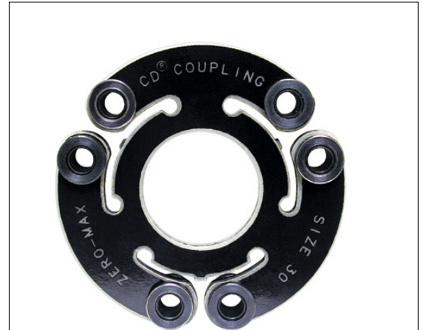
PHOTO FIVE AND ILLUSTRATION ONE CAPTION: CD® coupling disc pack (above). The coupling transmits torque between shaft coupling hubs similar to any conventional coupling. Yet the disc provides greater flexibility, misalignment, longer life, and damps shock and vibration through its unique patented open arm design with the use of highly durable composite material.
