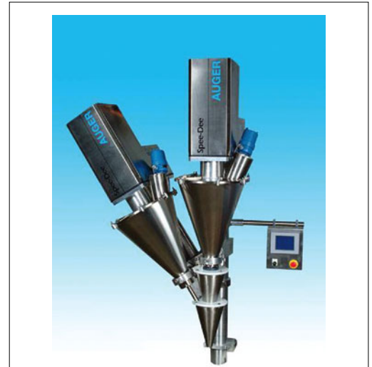
PHOTO ONE CAPTION: Spee-Dee Packaging Machinery, Inc. canted head dual auger system fills two dry food products with different characteristics through a single tube and into one pouch or package.
